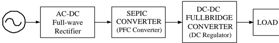
Figure 1. Block diagram of SEPIC converter and full- bridge DC-DC converter connected in series circuit
