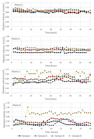
Figure 11. Vibration velocity profile
