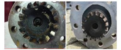
Figure 15. Deposit at No 1 Nozzle, after used Sample I (left side) and Sample III (right side)
