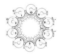
Figure 12. Combustor chambers [6]
