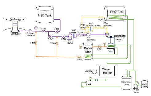
Figure 6. Sub-facilities of blending facility
