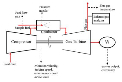
Figure 3. Flowchart of the experiment
